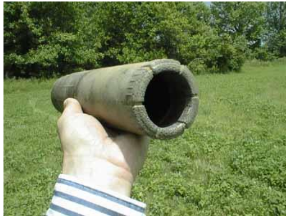
Figure 14. A diamond-tooth bit is used to advance rock core sampling. The bit grinds an annular ring allowing a sample recovery tube to slip around the rock core. Rock coring is several times the lineal foot cost of soil sampling.
