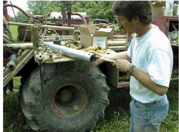
Figure 10. The driller estimates how much of the soil was recovered in the tube. This type of sampling is useful for getting relatively undisturbed soils in cohesive (silty and clayey) soil. It is very difficult to get samples in very rocky (too hard) or sandy (non-cohesive) soils.
