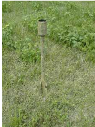
Figure 15. The vane shear test is used to attempt to get the shear strength of the soil in its natural, undisturbed test. This can be useful especially in soils where recovery is poor or there is concern that conventional sampling would disturb the soil excessively and make shear strength measurements in the lab unreliable.
