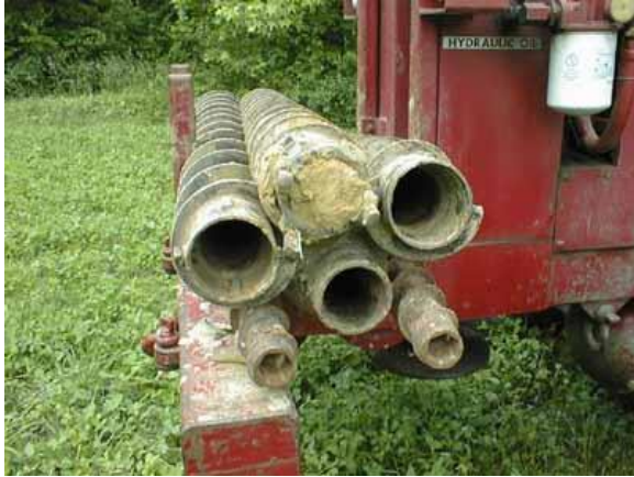
Figure 12. Augers of different configurations. The top four augers are hollow stem. The center-top auger has a plug with cutting teeth.
